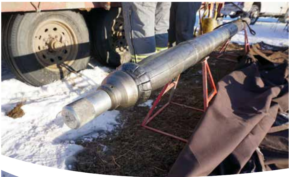
Casing expander tool, Liard East Field, February 2023. (Credit: OROGO)
