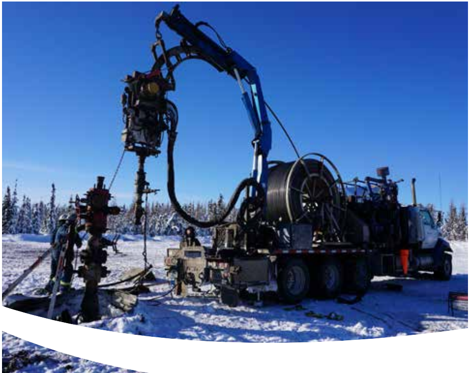
Coiled tubing rig, Cameron Hills, February 2023. (Credit: OROGO)
